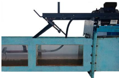
Figure 4. A view of the dynamometer used to measure the hydrodynamic coefficients of thrust and torque
