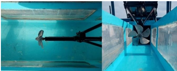
Figure 3. Front and top view of a surface piercing propeller in the test section
