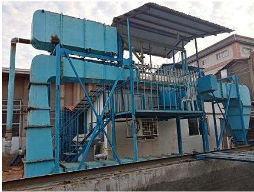
Figure 2. A view of the free surface water tunnel of Noshirvani University of Technology, Babol, Iran [18]
