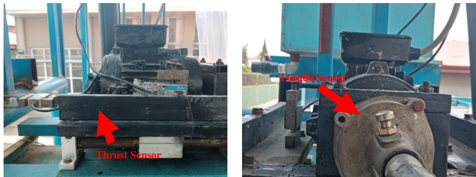
Figure 5. Location of thrust and torque sensors
