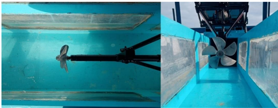
Figure 6. View of the impeller installed in the test section
