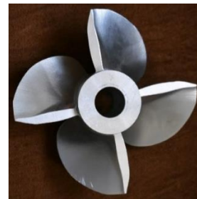
Figure 10. Model propeller made based on the characteristics of Olofsson [2] propeller with a diameter of 125 mm
