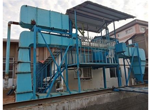
Figure 3. Free surface water tunnel of Hydrodynamics and Marine Propulsion Research Lab. in Sea-Based Energy Research Group, Babol Noshirvani University of Technology
