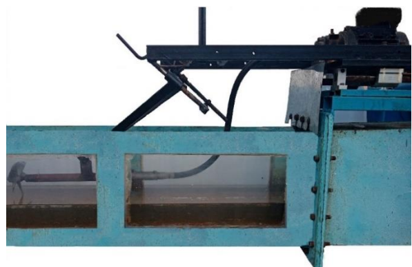
Figure 4. Overview of dynamometer with model propeller in the test section
