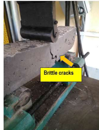
Figure 14. The brittle-like pattern of crack for bamboo reinforced beam
