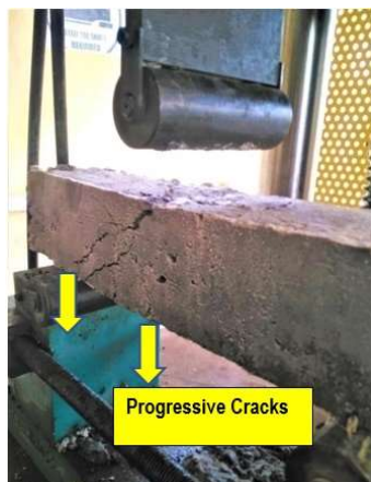
Figure 13. The progressive-like pattern of crack for steel reinforced beam
