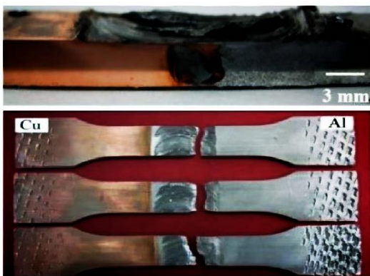
Figure 6. Optimal sample of weld number 7 after surface finishing operation
