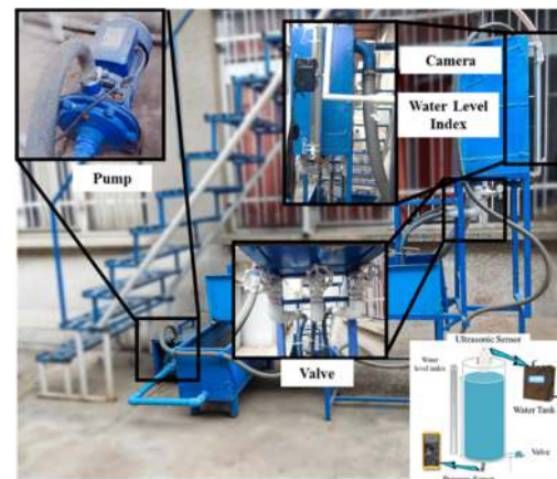
Figure 8. Using tank, camera, and ruler to calibrate the wave gauge sensor
