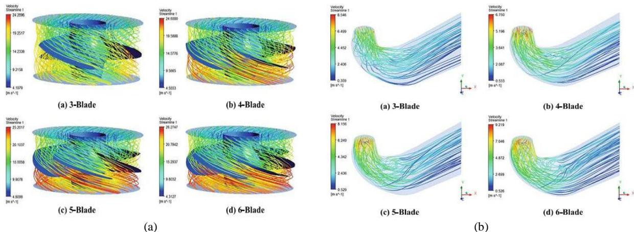
**Figure 4.** Sreamline in runner different solidity simulation at (a) runner (b) drafttube [21]
