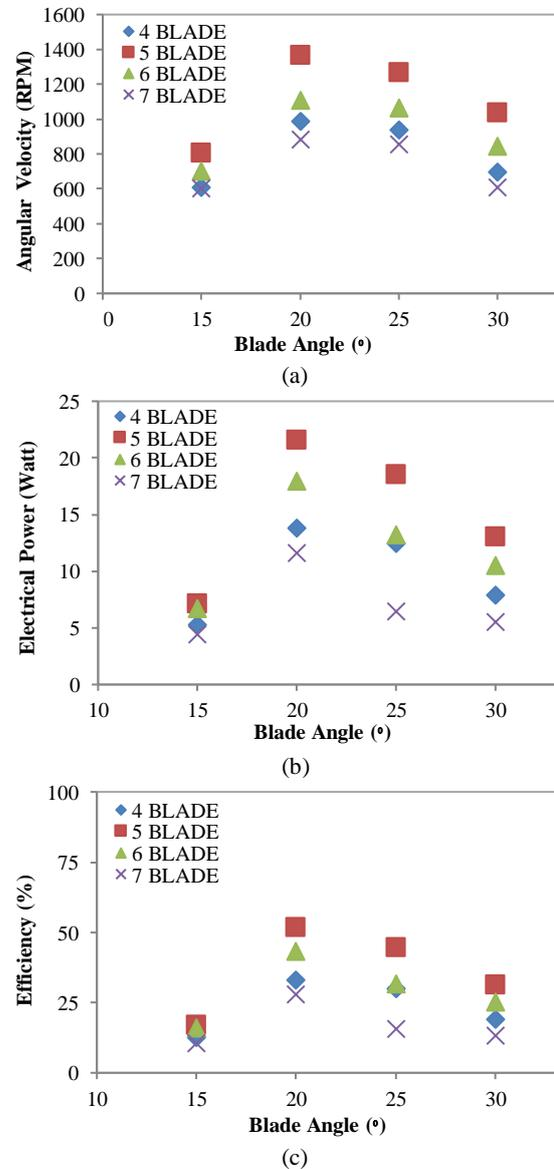
**Figure 3.** Relation between blade angle with (a) angular velocity, (b) electrical power, and (c) efficiency
