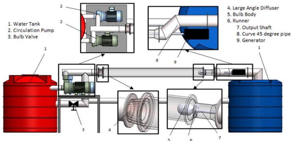
**Figure 2.** The sketch of rig test
