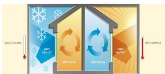
Figure 2. Low emission glass mechanism in winter and summer (The visible beam passes, the winter heat is reflected inside, the summer heat is reflected outside)
